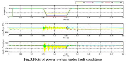
It is clear from the plots that there is a huge dip in voltage during the fault conditions and wild fluctuations of active and reactive power. This leads to system instability which may cause the machines to loose synchronism.
