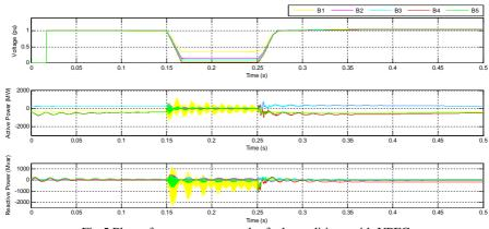
Fig.5.Plots of power system under fault conditions with UPFC
