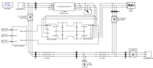
Fig.4.Power system under fault conditions with UPFC
